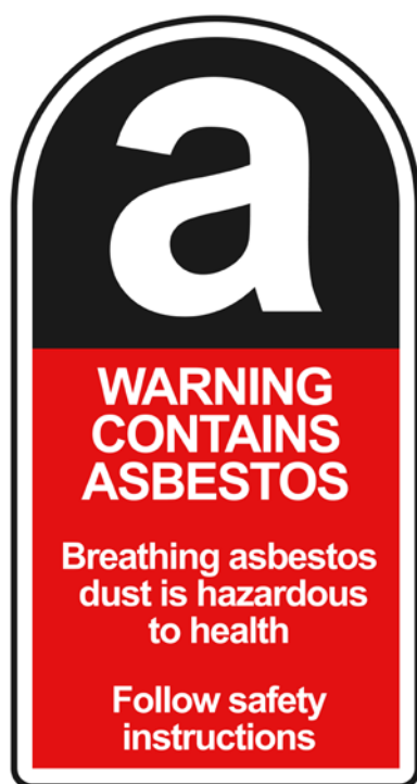
Figure A12-1: 'Warning contains asbestos' label
